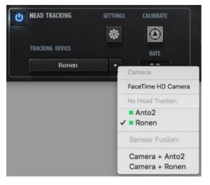
CAMERA activates computer's camera for head tracking. If more than one camera is available, choose from the list.
