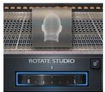
The **Rotate Studio** wheel rotates the studio around your position at the mixing desk. What you see and what you hear are defined by your orientation. This is what you experience when using head tracking, except that Rotate Studio is controlled manually.
