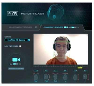
ON/OFF SWITCH lets you turn camera tracking **on** for tracking or **off** to save CPU resources. *This switch corresponds to the Head Tracking On/Off switch on the plugin.*
